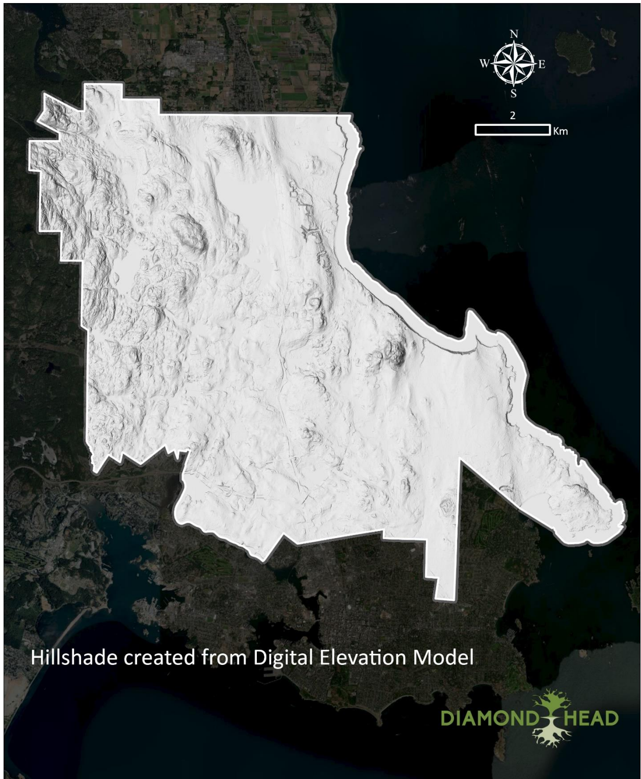
Figure 3. Digital Elevation Model of Saanich. This model can be used to develop contours and shows elevation across Saanich. It was derived from LiDAR and provided by the CRD.
